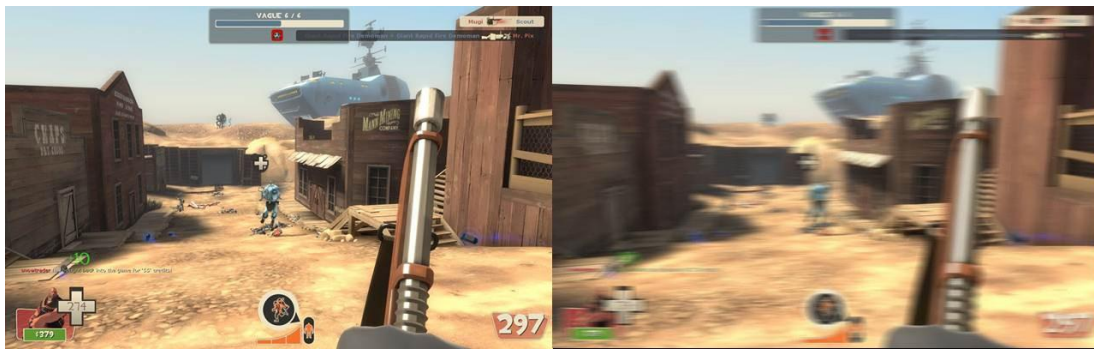
Figure 7 - Illustration of a 2 degree judder smear
