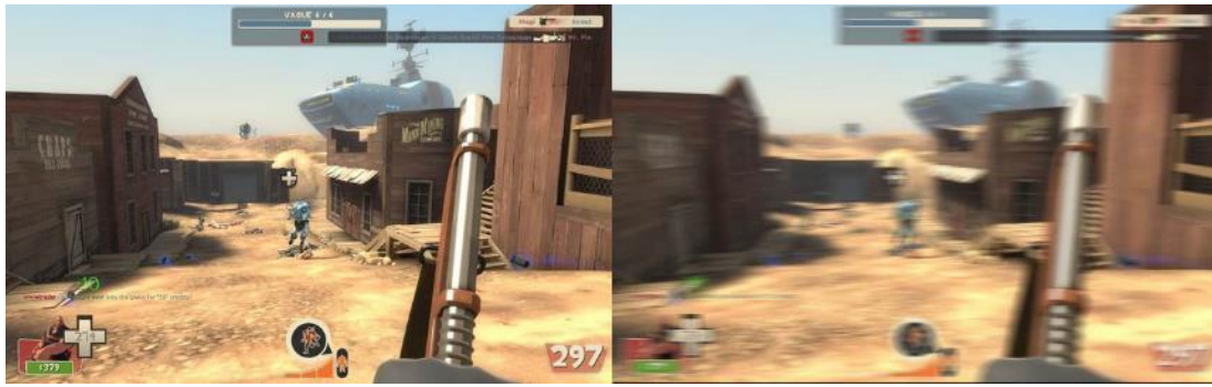
Figure 7 - Illustration of a 2 degree judder smear
