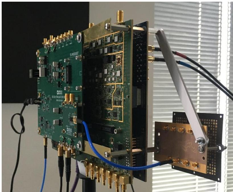
**Figure 39: 60GHz patch antenna and focussing lens**
